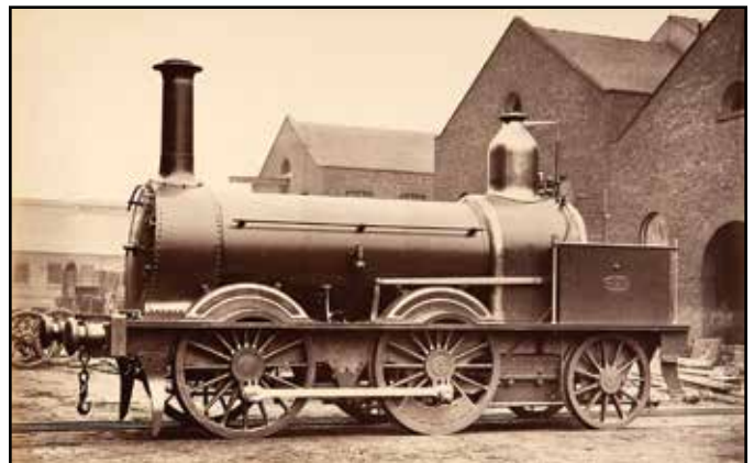
Beyer, Peacock and Company. Madras Railway (India) '0-4-2' tank locomotive Order No 425, 1860
